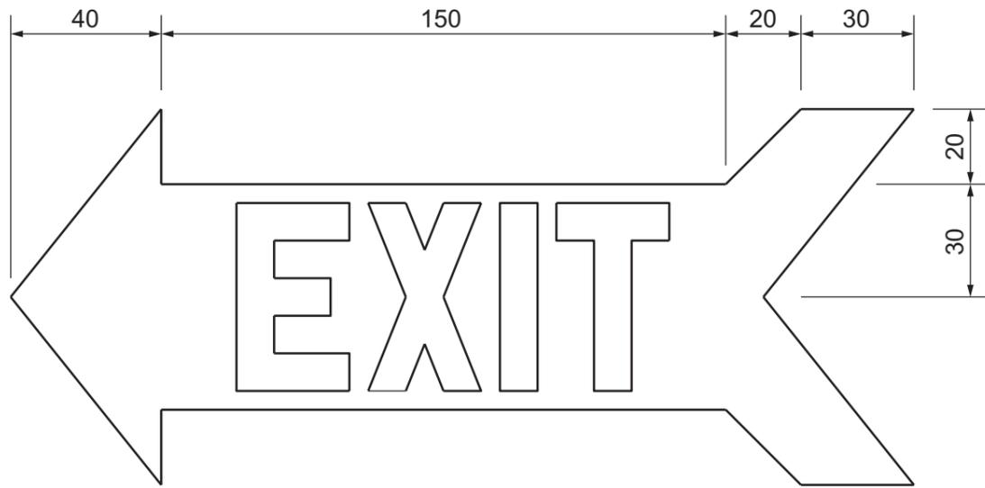
**A1** Complete the full size isometric view of the exit sign in the space provided to the right by drawing:
